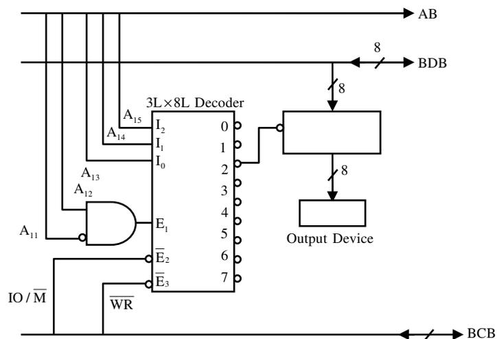
The interfacing circuit makes use of 3 Line to 8 Line decoder having 3 enable lines  $E_1, \bar{E}_2, \bar{E}_3$ .
