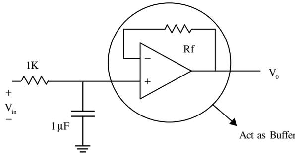
The given circuit is LPF (Low Pass Filter)
