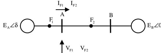
If the fault takes place at location  $F_1$ , then the voltage and the current at bus A are  $V_{F1}$  and  $I_{F1}$  respectively. If the fault takes place at location  $F_2$ , then the voltage and the current at bus A are  $V_{F2}$  and  $I_{F2}$  respectively. The correct statement about voltages and currents during faults at  $F_1$  and  $F_2$  is
