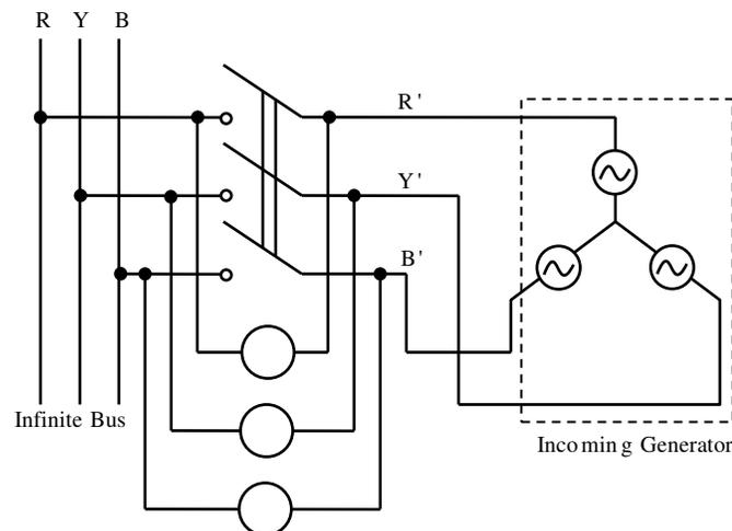
It was found that the lamps are becoming dark in the sequence  $L_a - L_b - L_c$ . It means that the phase sequence of incoming generator is
