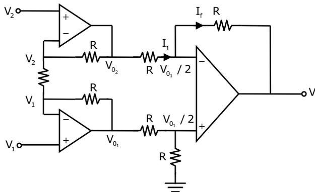
$$\frac{V_2 - V_1}{2R} + \frac{V_2 - V_{02}}{R} = 0 \quad \left| \quad \frac{V_1 - V_2}{2R} + \frac{V_1 - V_{01}}{R} = 0 \right.$$
