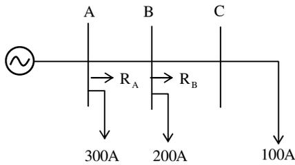
$$t_{op} = \frac{0.14 \times T.M.S}{(P.S.M)^{0.02} - 1}$$
