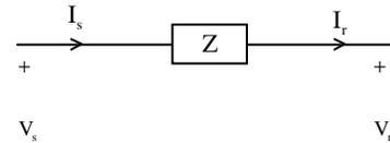
$$\begin{bmatrix} V_s \\ I_s \end{bmatrix} = \begin{bmatrix} A & B \\ C & D \end{bmatrix} \begin{bmatrix} V_r \\ I_r \end{bmatrix} \quad \begin{matrix} V_s = V_1 \angle 0, B = 0.1 \angle 90 \\ V_r = 1 \angle \delta_2, A = 1 \angle 0 \end{matrix}$$
