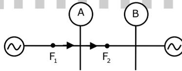
Current is feeding into the BUS A. It is like a generator delivering power to Bus (A)
