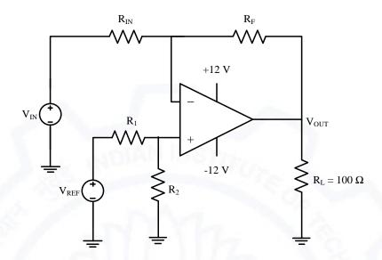
If  $V_{\rm OUT}=1$  volt for  $V_{\rm IN}=0.1$  volt and  $V_{\rm OUT}=6$  volt for  $V_{\rm IN}=1$  volt, where  $V_{\rm OUT}$  is measured across  $R_{\rm L}$  connected at the output of this OPAMP, the value of  $R_F/R_{IN}$  is
