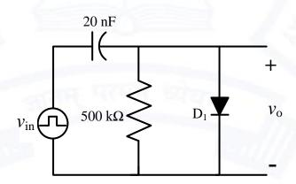
The difference between the maximum voltage and minimum voltage of the output waveform  $v_0$  (in integer) is \_\_\_\_\_\_ V.
