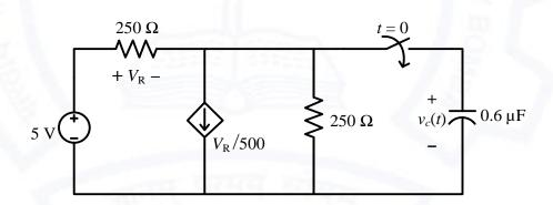
The time after which the voltage across the capacitor becomes zero (rounded off to three decimal places) is \_\_\_\_\_ ms.
